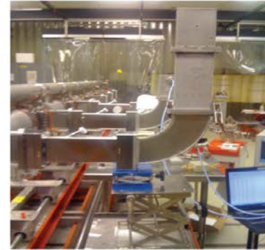
existing JLab 1.5 GHz coupler waveguide tested for up to 13 kW CW
