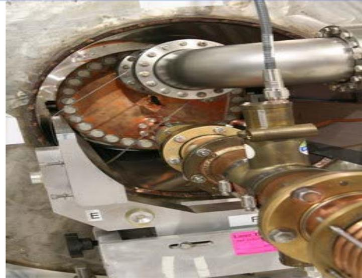
Cavity installed in bore of superconducting magnet in the MTA
